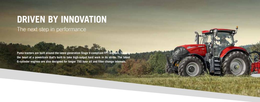
The 6.7 litre 4-valve engine with Common Rail high-pressure fuel injection and wastegate turbocharger delivers performance, torque, fuel efficiency and reliability between 140 and 180 hp (rated). All models benefit from an Engine Power Management boost for PTO, hydraulic and transport work, taking those figures to 175 to 225 hp.
