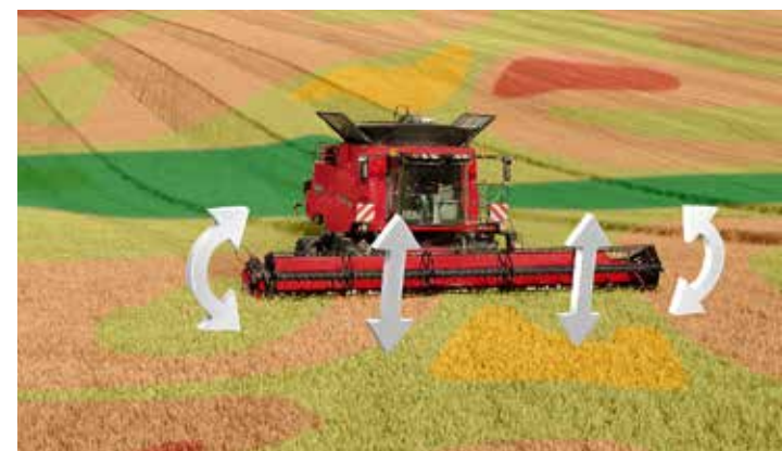
Case IH Terrain Tracker technology ensures that an exact cutting height is maintained across uneven fields.
