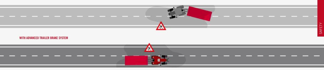
The Advanced Trailer Brake system actively recognises the current driving situation and stabilises the tractor and trailer combination by using the trailer's brakes.
