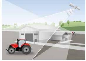
xFill bridges RTK<sup>+</sup> signal losses of up to 20 minutes
