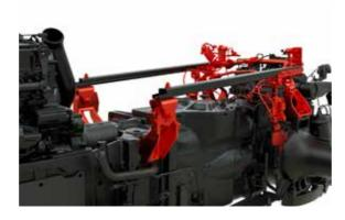
The semi-active, hydraulic cab suspension reliably absorbs jolting and vibrations.
