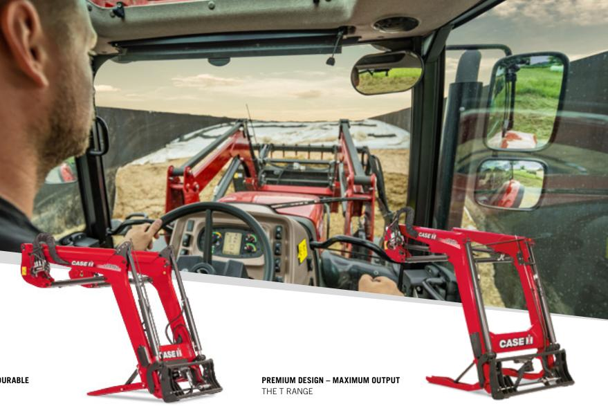
• Maximum lift heights from 3.76 m up to 3.90 m • Maximum lift capacities from 1,894 kg up to 2,327 kg
