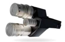
Oil motors or implements making large demands of the hydraulics can be supplied with up to 110l of oil per minute via the Power Beyond connection.
