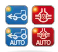
Easy-to-use buttons for all-wheel-drive and differential lock on the ICP control pad.
