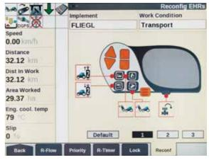
ISOBUS functions can be configured onto existing controllers such as the Multicontroller, joystick and control levers.
