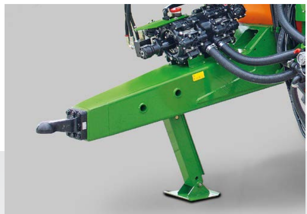
Lower mounted drawbar with towing eye and mechanical parking jack
