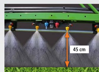
80° nozzles: 25 cm nozzle spacing
