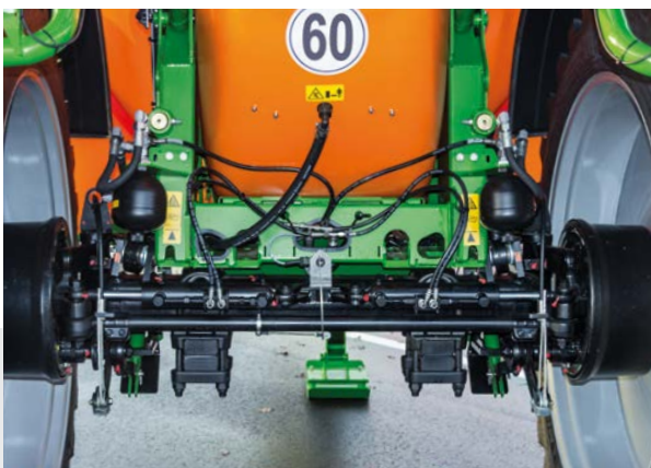
Hydro-pneumatic axle suspension with AutoTrail axle steering
