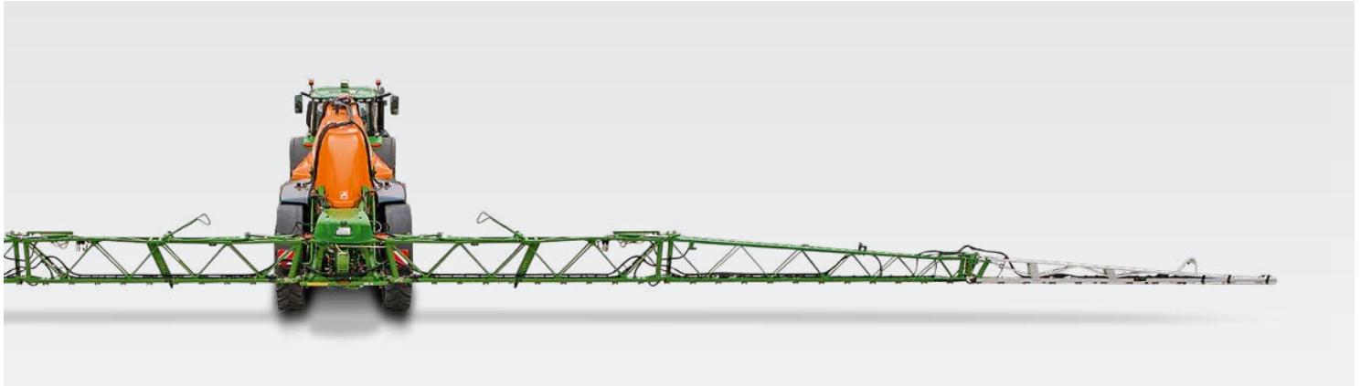
UX 11201 Super with 36 m Super-L3 boom
