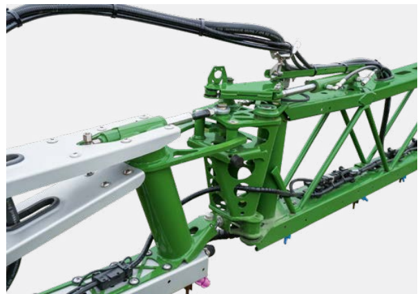
36 m Super-L3 boom, usable at both 24 m and 12 m as well
