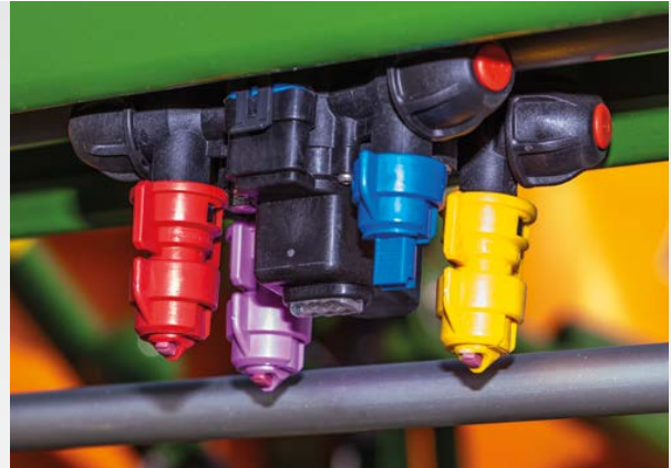
✓ AmaSelect electric individual nozzle control
