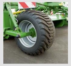
**Light treading and easy pulling** The EasyCut 6210 CV models run on oversized wheels and 500/45-22.5 tyres in standard configuration. These have proven best in soft terrain.
