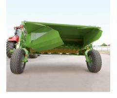
**Perfect double swaths** The long and pivoting swath boards tighten the material flow and present a fluffy swath.
