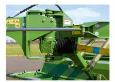
**Frictional connections without belts** The drive power flows via overload protected gearboxes and drive shafts to power the cutterbar and conditioner. Two slewing gearboxes optimize the power flow down the drive shafts.
