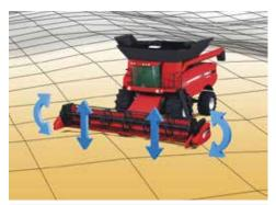
Case IH Terrain Tracker technology ensures an exact cutting height is maintained across the most uneven of ground.
