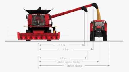
**Standard unloading system** at 113 l/s suited for grain and corn headers up to 12.5 m width High capacity unloading system at 141 l/s for 7240 and 8240 or 159 l/s for 9240 combines for grain and corn headers up to 12.5 m width
