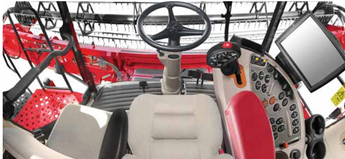
Comfortable cab, full view of the header and ergonomically laid-out control console
