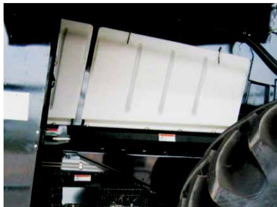
Outstanding maintenance access from left hand side by removing moulded white plastic covers
