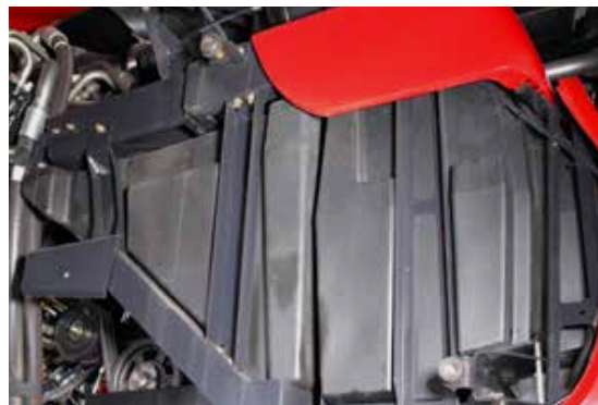
Fuel capacity of 1,125 litres (7250, 8250) or 1,200 litres (9250) for long working days. When equipped with the Xtra-Chopping chopper, the 9250 has a capacity of 1020 litres
