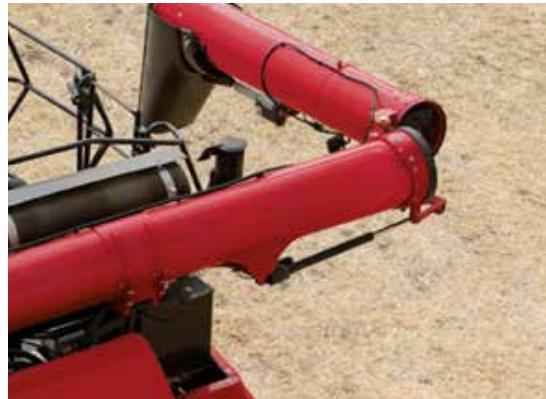
The 8.8 m and 10.4 m unloader augers are available as foldable versions for easier transport on the road and for easier manoeuvring in sheds for storage
