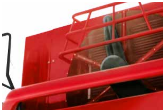
Fixed radiator grille for optimal dust clearing
