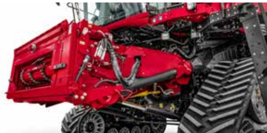
Fore-aft tilting for setting of header angle – all laid crop picked up, minimal losses
