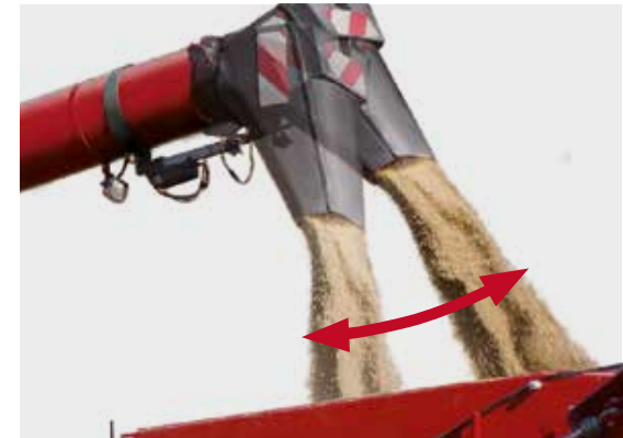
The pivot spout option is operated with the multi-function handle and directs the grain stream into the grain cart, filling it without spillage to maximum level
